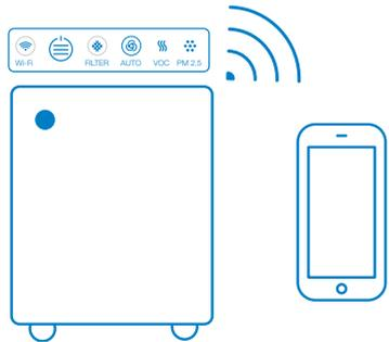
The air purifier can also be automatically regulated based on the air quality readings from the built-in sensors (680i), or the optional external air quality monitor Blueair Aware™ (605, 505)
