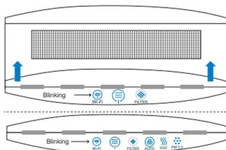
Open the flip-up lid and press the air-flow speed touch button. When the Wi-Fi symbol starts to blink, the air purifier can be paired with the Blueair Friend mobile app.
