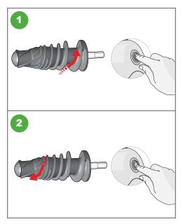
Press [Rev] button for 3 to 5 seconds, then release. When the [Rev] button is released, the auger will stop rotating. Repeat this 2 to 3 times.
